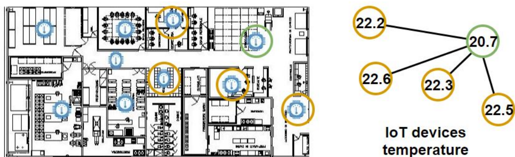
Figure 3. Smart building with an IoT network. The measurements from each device are sent to a consensus algorithm to be processed. There are five IoT temperature measurements, four from accurate IoT devices (orange), and another one from an inaccurate IoT device.
