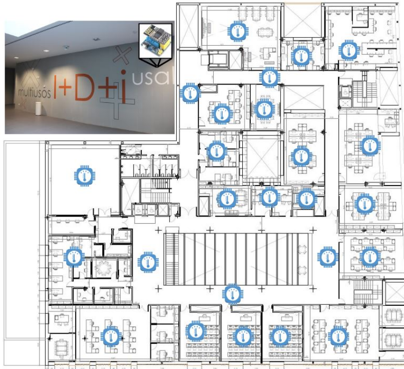
Figure 4. Map of the case study building. In this figure, IoT device location in the smart building is displayed.
