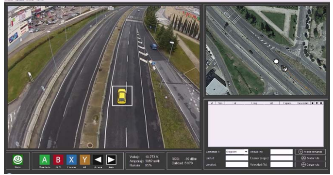
Fig. 3. Screenshot of the developed software during a flight where the yellow car (in the white frame) is the objective to track.
