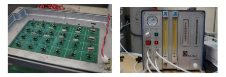
Fig. 6. Permeater and QCM sensors
