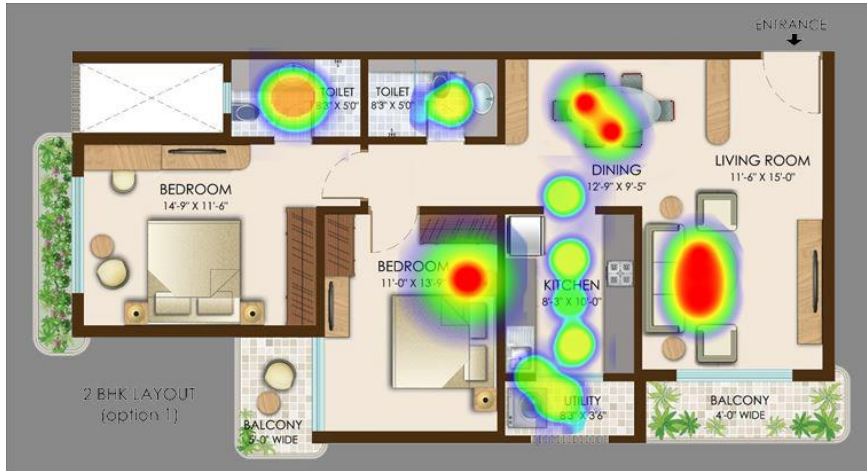
Fig. 3: Example of use of RTLS at home to determine positions and behaviors of users.
