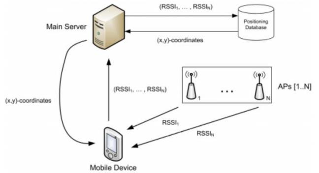
To deploy the solution localization and reduce costs, we used the actual hardware, leveraging existing routers whose model is TL-WR740N. The main advantage of this device is the ability to install a Linux-based firmware that allows us to run programs in script mode, in our case, we have replaced the factory version for DD-WRT based firmware.
