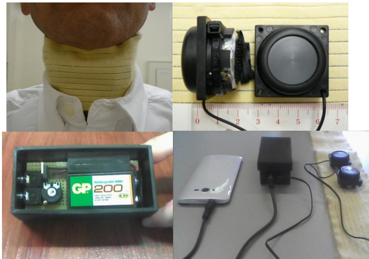
Figure 4: EL transducer, amplifier and entire system (upper left: EL transducer with neck-bandage, upper right: a pair of EL transducer, lower left: amplifier in a box, lower right: entire system)
