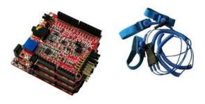
Fig. 2. Arduino Shield EKG-EMG and electrodes
