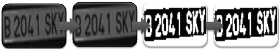
Fig. 2. Outlining the transformation of the image to identify the plate digits
